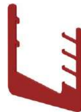
Support bracket hinged to support profile, to position conductor rails during installation
