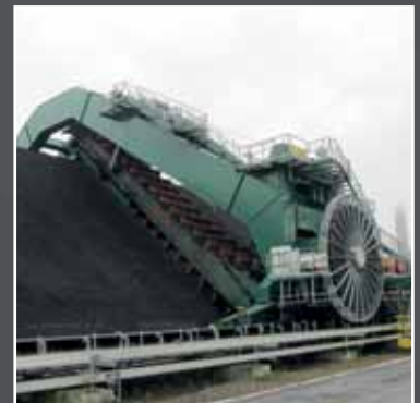
Motor Driven Cable Reel on a Portal Stacker, USA
