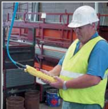
Push Button Pendant on an EOT Crane, Australia
