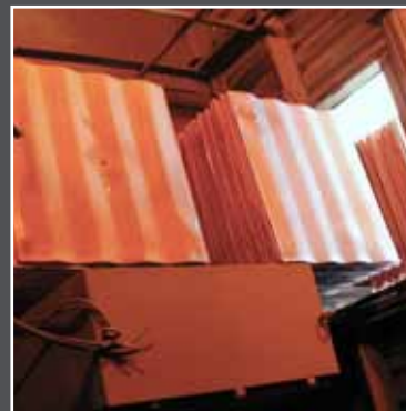
Finished Copper Sheets Coming Off the Line
