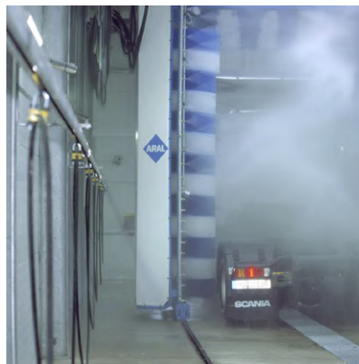
Hose-transportation in a truck washing facility
