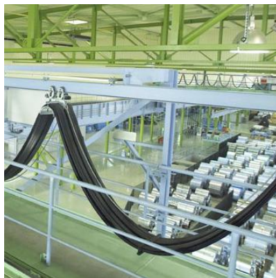
Energy and data transmission on a steel-mill-crane
