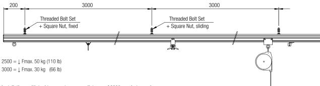
Installations with tool transporters, max. distance of 2000 mm between hangers:
