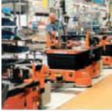
With IPT®-Floor powered vehicles in an axle assembly line
