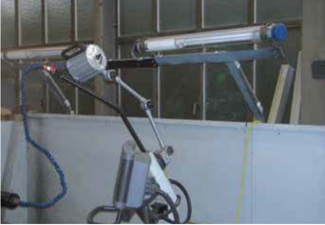
MasterLED - lathe workplace illumination
