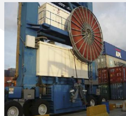
E-RTG (Plug-in-version) with cable reel solution
