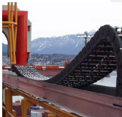
Standard energy guiding chain for RTG
