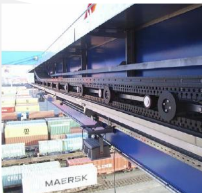
Energy guiding chain solution for trolley – Railway terminal, Weil am Rhein, Germany
