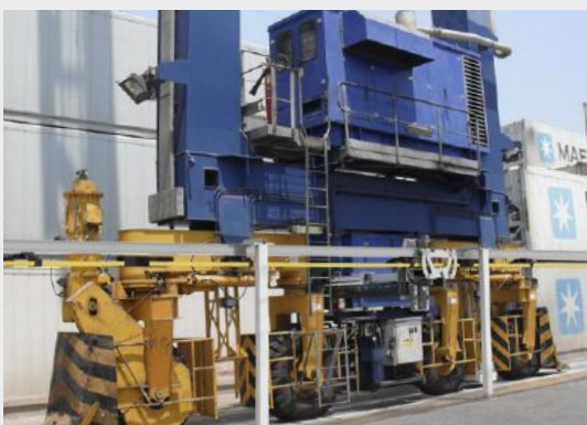
Conductor Rail "Drive-In" System for E-RTG
