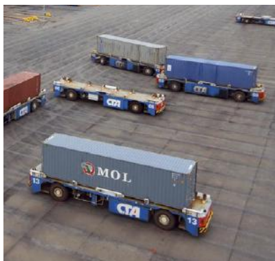
Fully automated AGV with electrical drives
