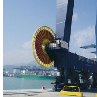
Medium-voltage motorized cable reel on STS Crane at YICT in China
