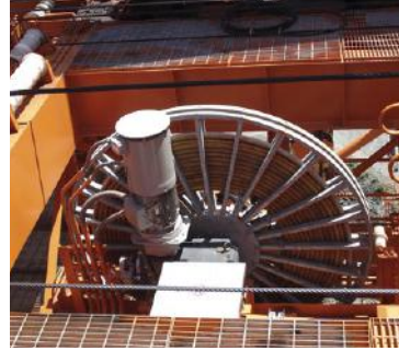
Motorized cable reel for spreader with variable frequency drive
