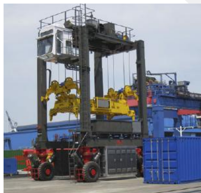
E-Straddle Carrier with Battery Charging Systems
