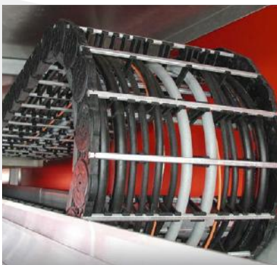
Energy guiding chain in guiding channel
