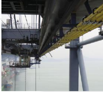
Conductor rails with inductive data transmission
