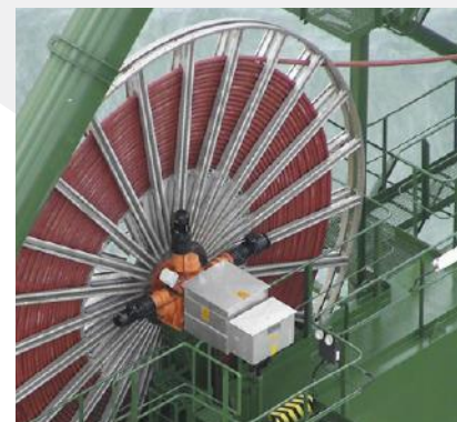
Medium-voltage motorized cable reel with magnetic coupler
