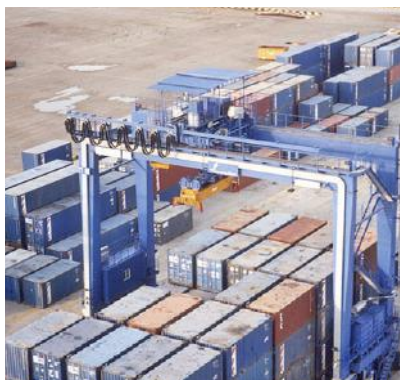
Standard festoon system for RTG-Main trolley
