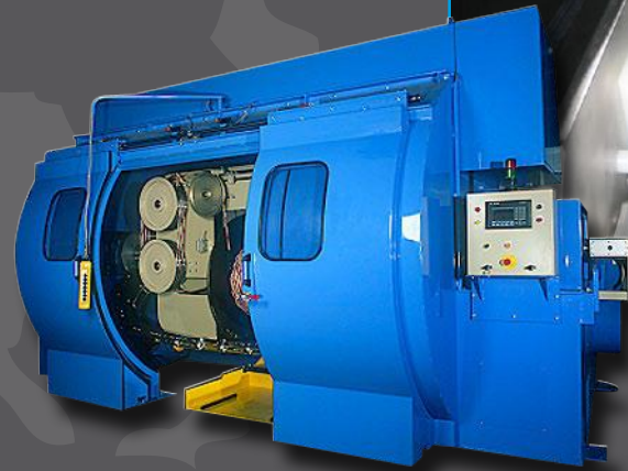
Rollertwist strander: a real Unilay
