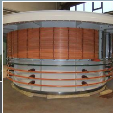
Slip Ring under construction 2200 mm Inner diameter, 4200 mm outer diameter
