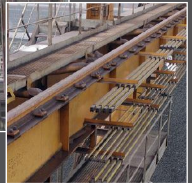
Conductor Rails on a tripper conveyor
