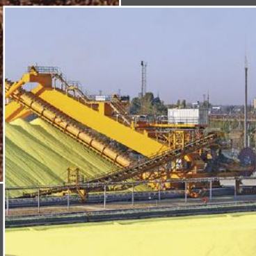
Monospiral Reel on a Portal Stacker, Russia Travel Length: 480 m
