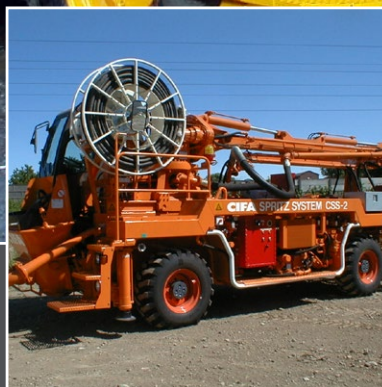
NAMI reel on shotcrete machine by Cifa
