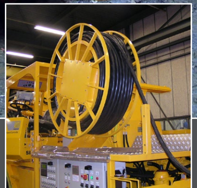
NAMI reel on shotcrete machine by Sika
