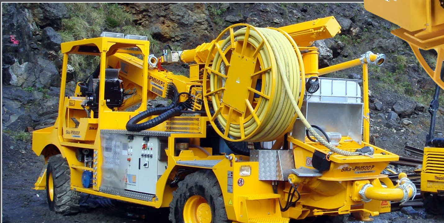
Hydraulic drive cable reel on shotcrete machine
