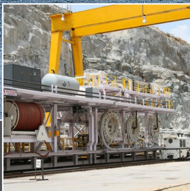
Orion cable reel on Tunnel Boring Machine by The Robbins Company
