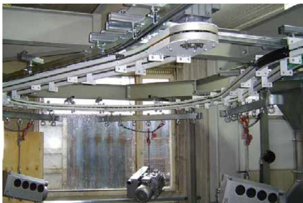
**Semiautomated C-rail system with overhead loop-conveyor**
