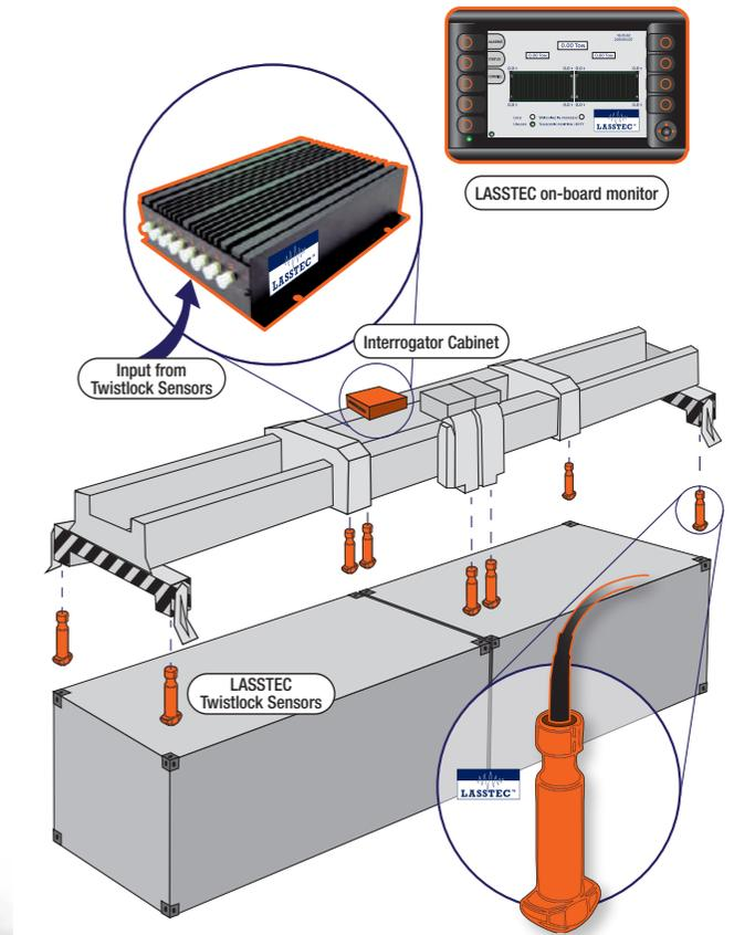
*The LASSTEC system is the first technology to measure the load “where it really happens”, namely directly on the spreader twistlocks.*
