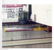
Wampfler's Buffer design incorporates the proven damping system of multiple orifice patterns drilled down the shock tube length, for precise deceleration profiles, coupled with a nitrogen return system for controlled extension of the piston rod to its original position.
