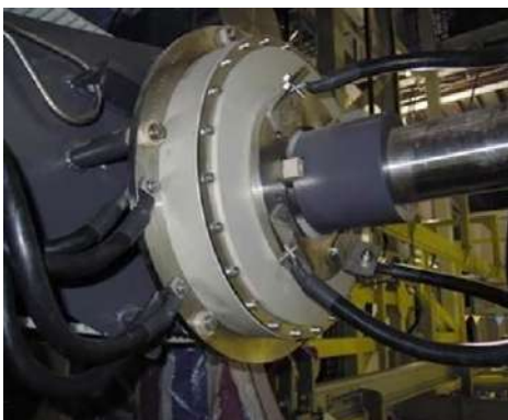
Slip Ring in an electrophoresis plant
