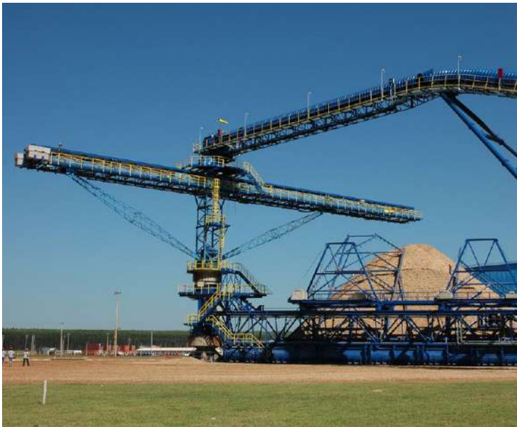
Stacker/Reclaimer with large bore slip ring
