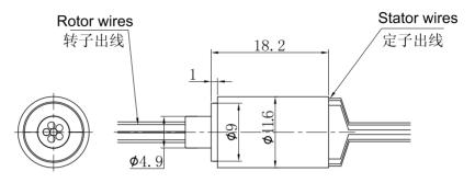
Rotor side Stator side 定子边
